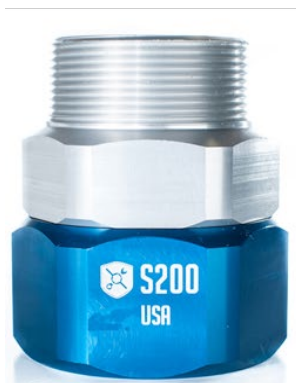
S200—BLUE ANNODISED BASE; 2.0" NPT THREAD; 2.0" FNPT BASE; HEX 3.0"; HEIGHT BASE TO TOP OF THREAD 3.54"
