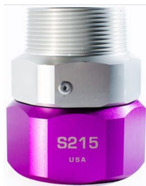
S215—PURPLE ANNODISED BASE; 2.0" NPT THREAD ; 1.5" FNPT BASE; HEX 3.0"; HEIGHT BASE TO TOP OF THREAD 3.54"
