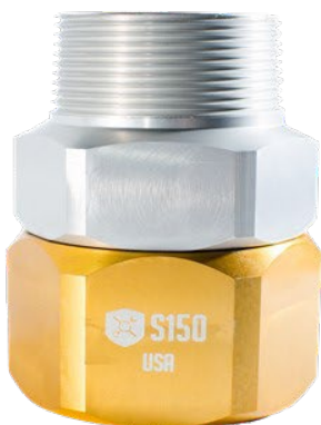
S150—GOLD ANODISED BASE, 1.5" NPT THREAD; 1.5" FNPT BASE ; HEX 2.38"; HEIGHT BASE TO TOP OF THREAD 3.54"
