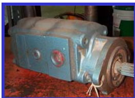
Gear main pump 1200-rpm P25X
