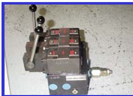
Floor jack manifold. (Jack-Safe) HYDEN125
