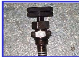
Cable reel motor bypass needle valve. HYDEN110-D
