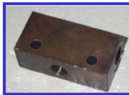
Dual service brake shuttle valve. HYDEN188
