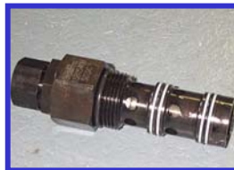
Boom cylinder load hold Set to suit Kis 2500-psi HYDEN269-A
