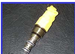
Cable reel pressure sensor. HYDEN110-A
