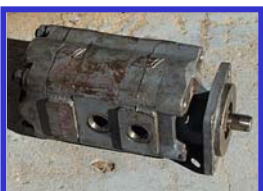
Gear main pump P30C
