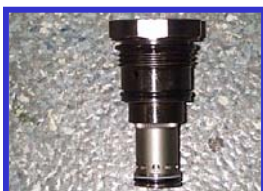
Boom main relief valve. HYDEN110-H
