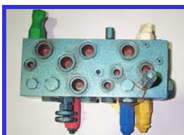
Pressure control manifold. (Kis block) HYDEN110
