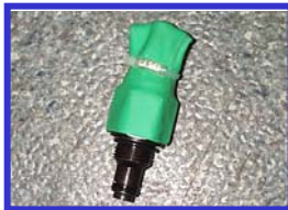
Boom pilot relief valve. HYDEN110-G
